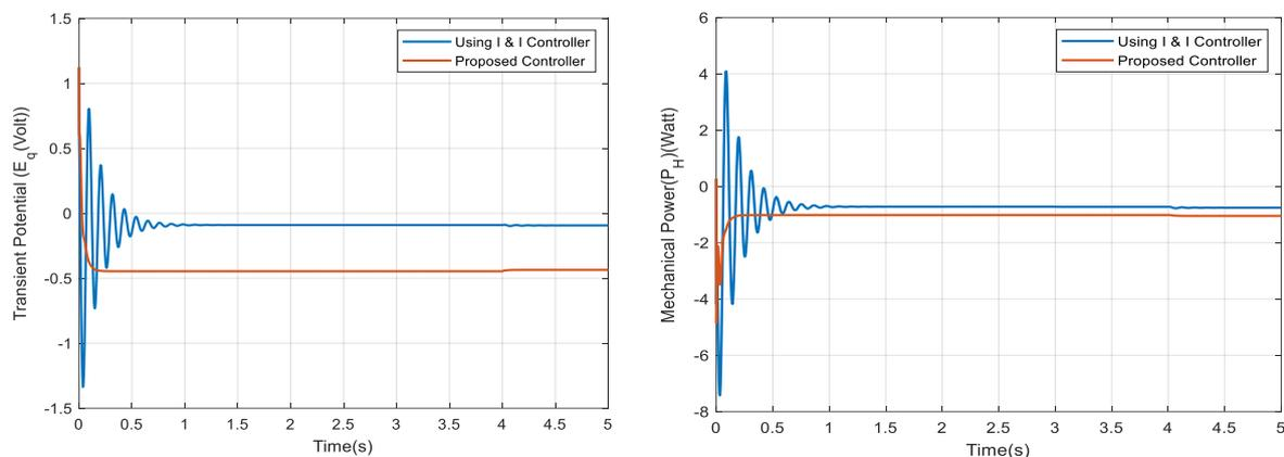
Figure 7(a): Comparison of the Transient Potential Stability (b) Change in Input Mechanical Power
