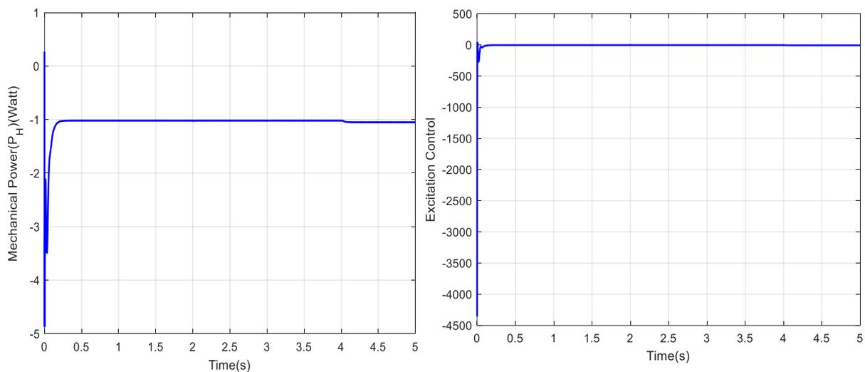
Figure 3(a): The Change Input Mechanical Power (b): Excitation Control of Proposed Controller
